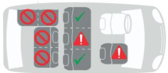
Do not use vehicle seats, which are arranged to side ways. These seats are not permitted to use for child car seats.
