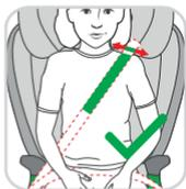
The diagonal belt should be centred over the child's shoulder, the lap belt should run as low as possible over the groin. Make sure that the diagonal strap is straight and not too close to the child's neck. All straps must be tight against the child's body and must not be twisted.
