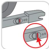
Check the safety indicators (IT). These must both be RED. If the safety indicators (red) are not visible, press the green release tabs until you hear an audible << CLICK >>.
